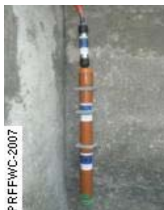
Digital Short-Messaging-System (SMS) enabled rain gages such as the one shown below are preferred for real-time observation in a CBFFWS.
