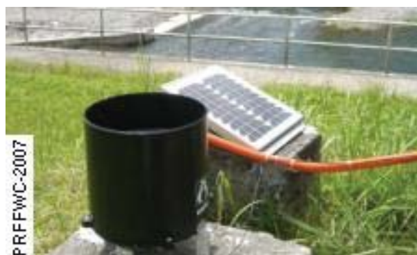
Digital Short-Messaging-System (SMS) enabled rain gages such as the one shown below are preferred for real-time observation in a CBFFWS.
