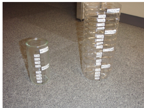
Fig 2.5.6 Simple precipitation gauges made of a glass and a plastic bottle
