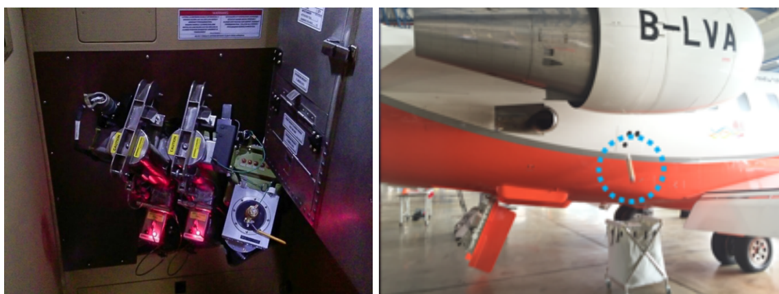
Figure 1 The meteorological profile measurement system (“dropsonde launcher”, left) inside the GFS Challenger aircraft, from which the dropsonde is launched during a ground test (right).
