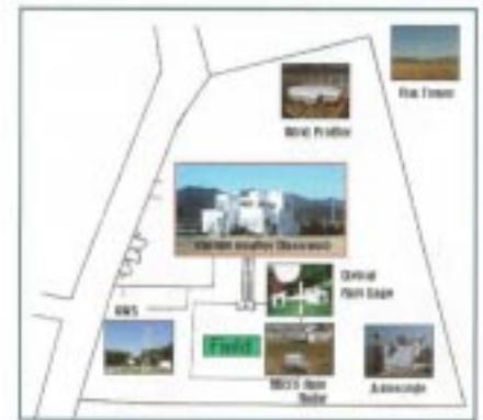
Arrangement of meteorological instruments installed at the National Center for Intensive Observation of Severe Weathers.
